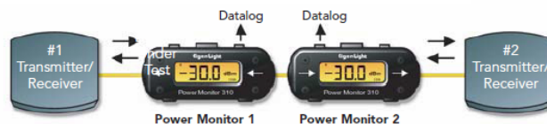
Monitor 1 Reading = Optical Power Delivered to Receiver #1 Monitor 2 Reading = Optical Power Delivered to Receiver #2
